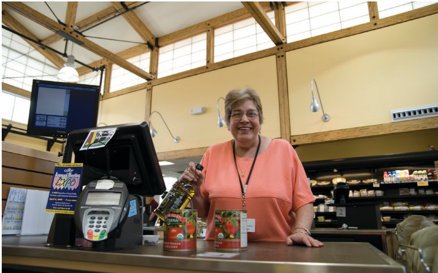
Linda Willson at the new Community Market. Passive sunlight fills the sales floor without glare, thanks to the Kalwall insulated and translucent panels.
